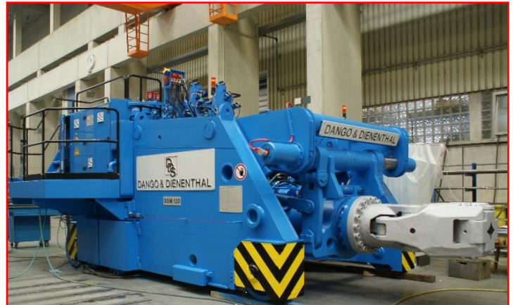
15 mt Railbound Forging Manipulator installed at 25 MN Open-Die Press for Light Metal products in Romania and China.
