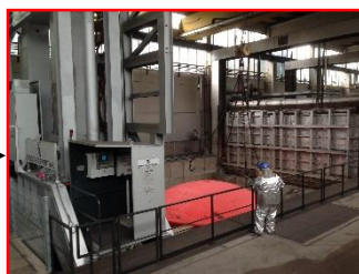
Fully automated Heat Treatment Line installed in a German Forge.
