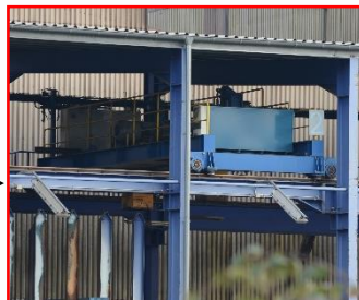
Fast overhead Bar Handling System in a stock yard at a German steel mill.
